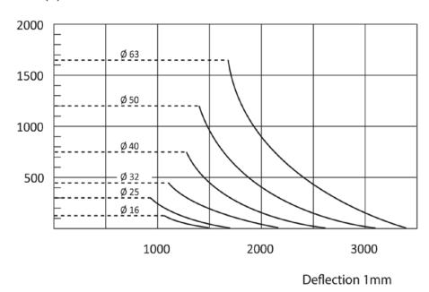
max. distance (SL) in mm - without mid section support / mid section mounting
